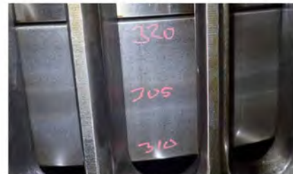
Light barrel shape skirt wear
