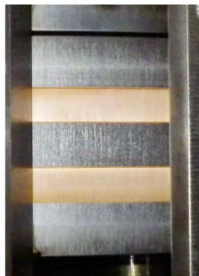
Bronze bands worn flush, but chamfers in fine condition.
