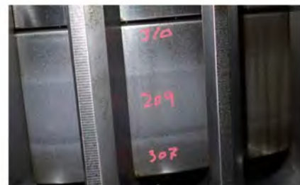
Moderate barrel shape skirt wear
